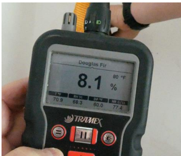
Measurement taken again and found dry plaster skim applied over wet wall. The area above bunk beds showed damp risk on IR but low on conductive meter at
