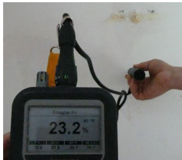
Measurement taken again and found dry plaster skim applied over wet wall. The area above bunk beds showed damp risk on IR but low on conductive meter at
