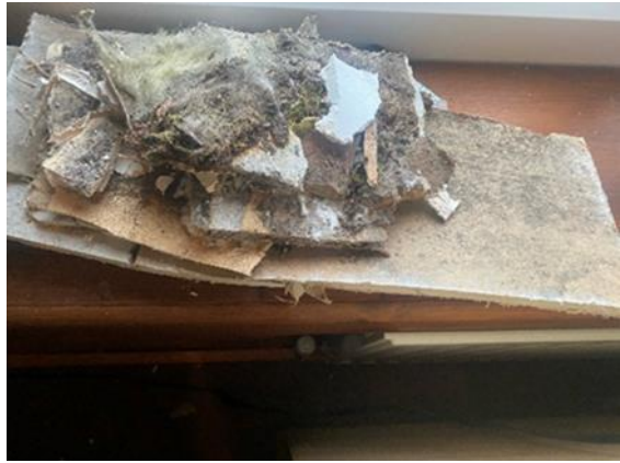
Visible mould to kitchen cabinet and ceiling removed during Pure Maintenance process Photos provided by client
