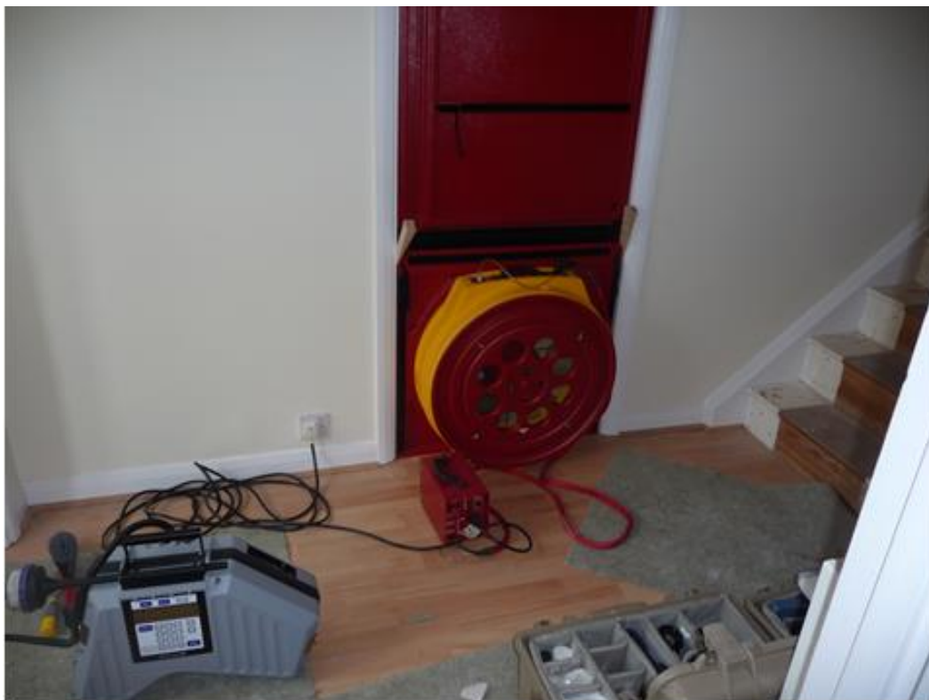
43 Negative Pressure blower door fitted to front door and produces negative pressure to property thereby exposing leaks
